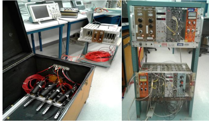
Figure 2: PMTs in dark box (left) and NIM electronics test setup (right)
