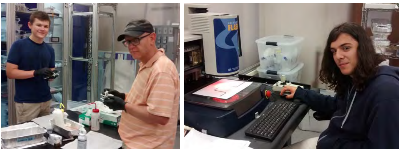
Fig 3: (Left) Justin Shute and Josh Owens working on end-of-stave mounts for the UT detector. (Right) Liam Meisner measuring the quality of the bending of the cooling tubes that will be embedded in the UT staves.
