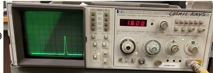
This reading shows the 1.6 GHz signal, ran through cable St 9 as - 41 dB.
