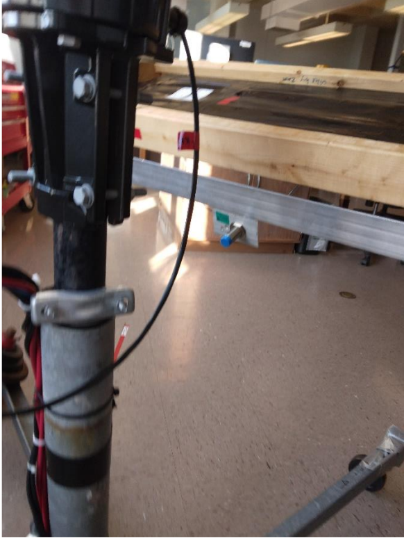
Left pic: small blue proximity sensor shown mounted on telescope frame
