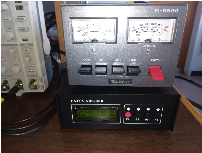
Yaesu G-5500 Elevation/Azimuth Controller to rotate axes (top), and EATX ARS-USB controller (bottom) to stream astronomical coordinates from computer (using NOVA for Windows) to Yaesu controller
