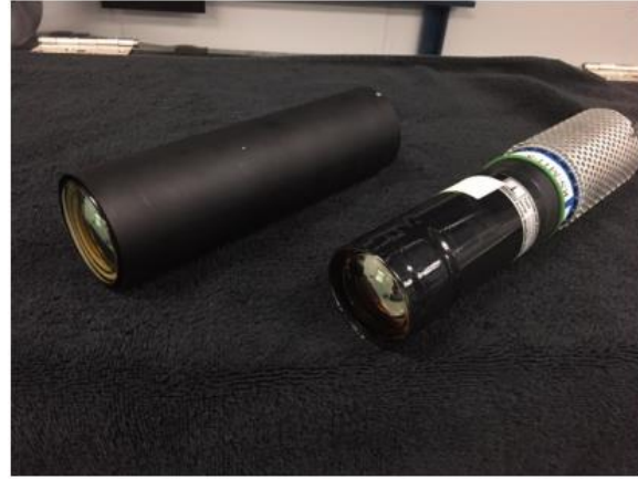
FIG. 2: A Hamamatsu tube Model Number H2431-50 on the left and an EMI tube Model number 9954KB05 on the right.
