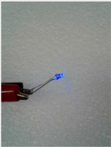
FIG. 3: Blue LED used to test PMTs
