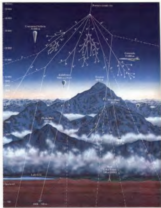
Figure 1. A cosmic ray shower produced by a primary cosmic ray entering the earth's atmosphere.
