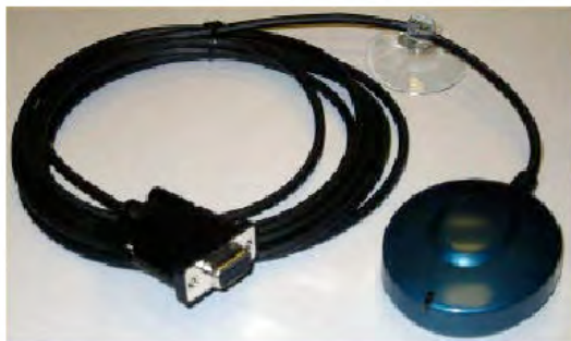
Figure 9. The LeadTek GPS receiver and cable. The cable shown here can be connected to a GPS extension cable.
