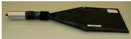
Figure 11. A typical cosmic ray counter consisting of scintillator and light guide (the flat paddle region to the right), the PMT (black cylinder), and the PMT base (light-colored cylinder on the left end.)
