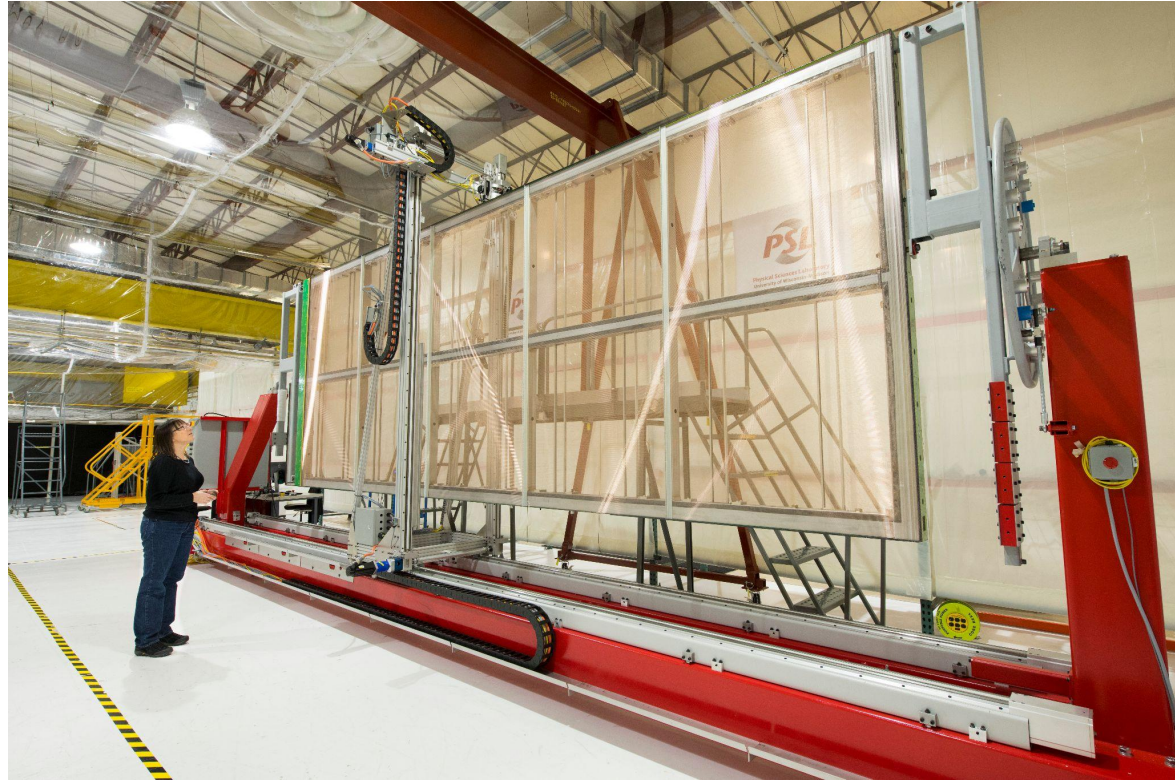
Wire planes to collect signal in a DUNE TPC
