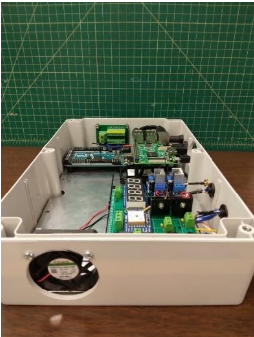
Fan side of the enclosure after cutout and holes drilled
