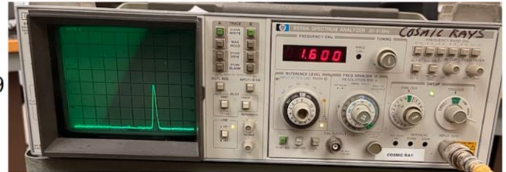
This reading shows the 1.6 GHz signal, ran through cable St 9 as - 41 dB.
