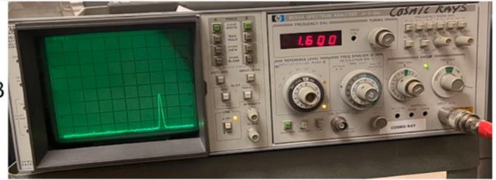
This reading shows the 1.6 GHz signal, ran through cable St8B as - 48 dB.
