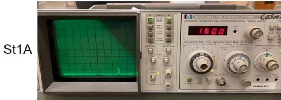
This reading shows the 1.6 GHz signal, ran through cable St1A as - 67 dB.
