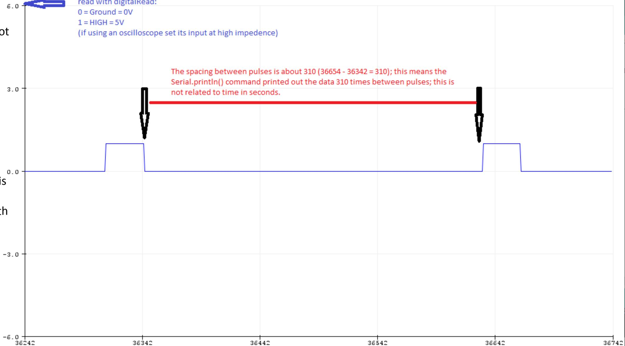
The serial plotter plot is correct; its horizontal axis represents the number of consecutive print lines from Serial.println(). The signal's time period cannot be interpreted from this plot, however it is clear the signal width is about 10% of the signal period.
