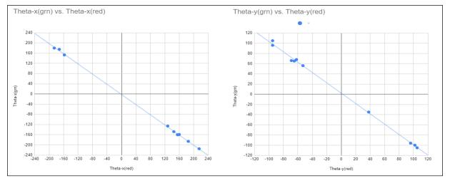
In these plots of green Xs vs red stars for  $\theta_x$  and  $\theta_y$ , respectively, note that the slopes are very close to -1 and that the vertical axis intercepts are very close to zero. The results, then, are very close to  $\theta_{x(red)} = -\theta_{x(grn)}$  and  $\theta_{y(red)} = -\theta_{y(grn)}$ . Also, note the gaps in the middle of the plots. The gaps show the region that is blocked by the beam pipe, which runs through the center of the detector.
