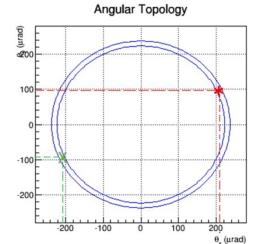
The event display shows a planar view, with the beam occupying an area in the middle; there is a gap in the detector there. The TOTEM detectors are embedded at the edges of the LHC beam pipe. Each records a "hit" where a scattered proton strikes. The red stars and green Xs represent these hits.
