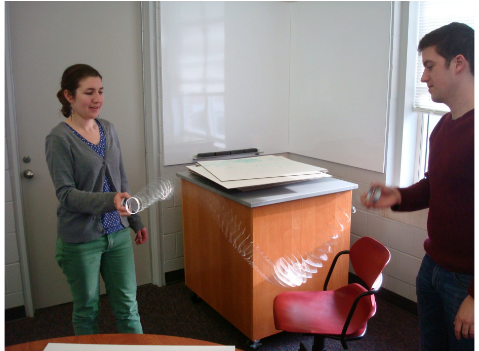
Wave propagation along a slinky
