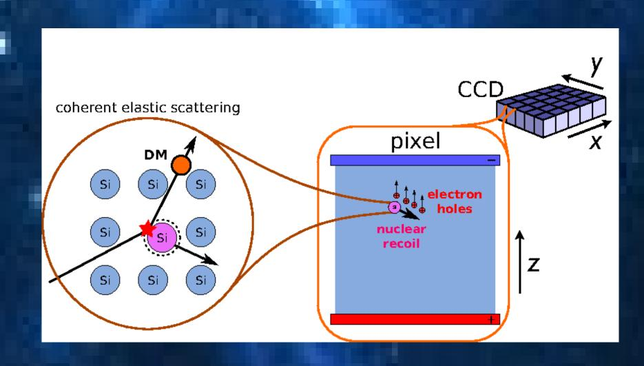
This image illustrates how the CCDs in the DAMIC experiment detect Dark Matter collisions. As DM interacts with nucleus of the Silicon through the weak force a flash of charge is produced, which is then recorded as an event.
